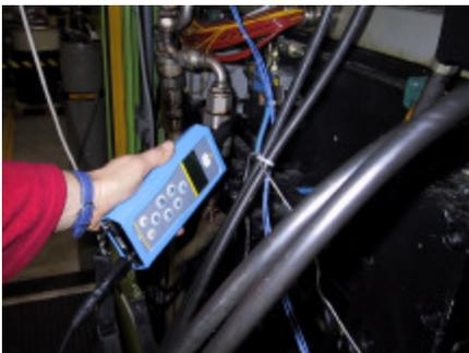
SDT has a line of accessories to address special situations in leak detection applications. A flexi-sensor allows the inspector to find leaks in tight or hard-to-reach areas. For distance capabilities, the Extended Distance Sensor (EDS) will allow leak detection at twice the distance capability of the
