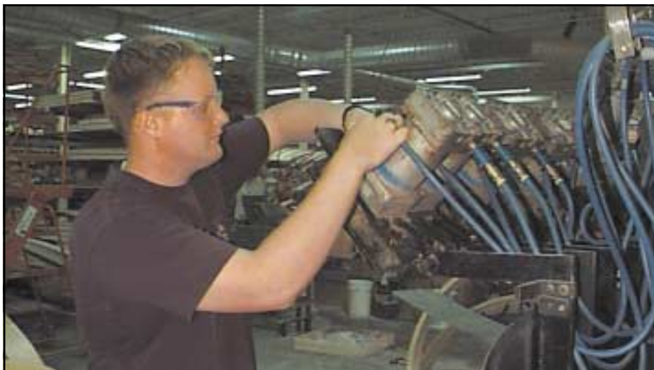
Randy Martens repairs leaky compressed air fittings on a radius clamp used to manufacture Loewen's line of arched windows.
