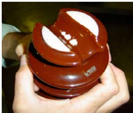
Figure 1 - The insulator shown here was damaged by tracking and eventually arcing.
